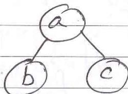
→  $a$ 's degree is 2 but  $\text{size}(a) = 3 < 4$  no. of nodes in  $a$ 's tree.
