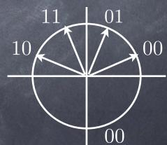
Extracting 2nd bit Rotate by  $\pi/8$ Measure
